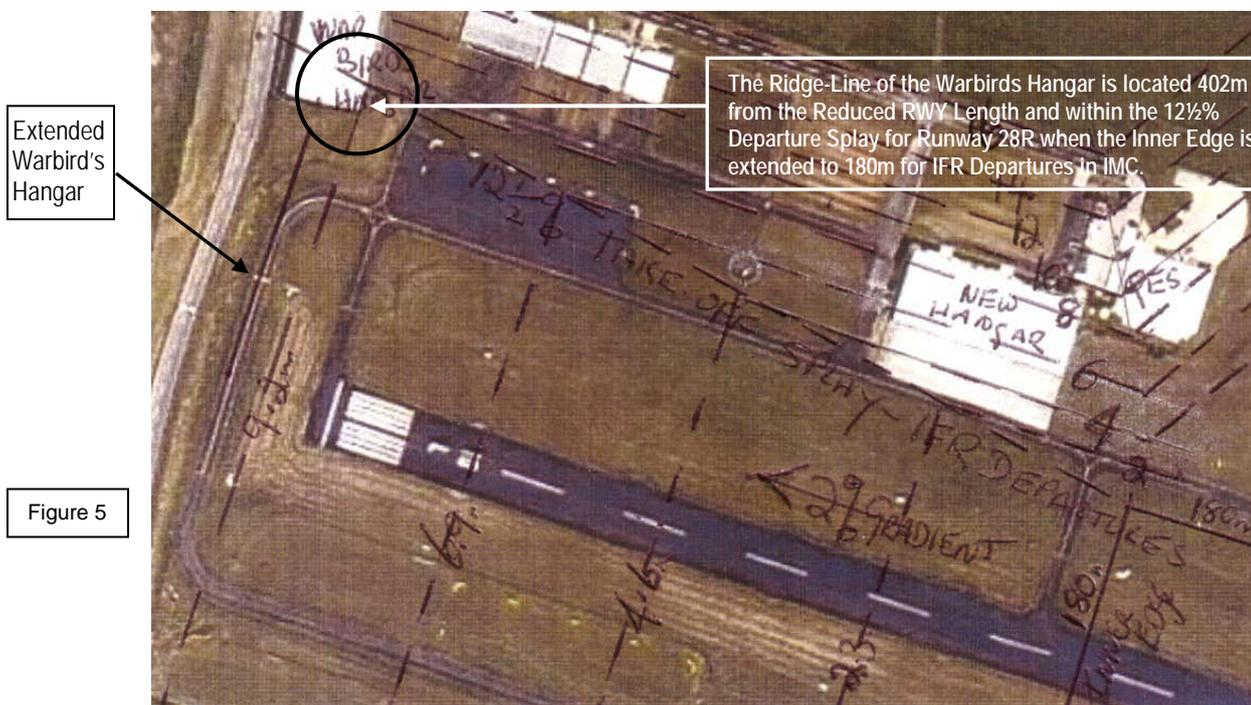
The Warbird's Hangar Roof is within the Take-Off Splay for 28R IFR Departures in IMC & Penetrates the 2% Gradient
